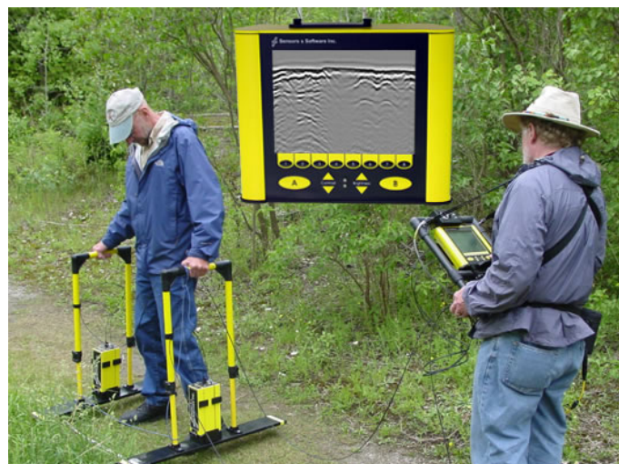
A pulseEKKO 100 MHz system deployed in bi-static step mode operation.
